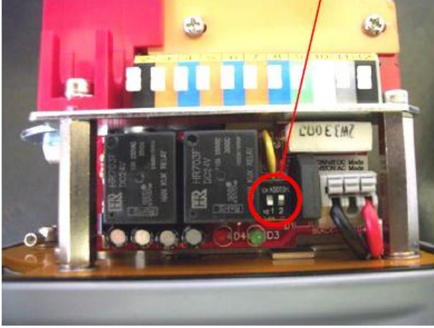
AC OPERATION DIP SWITCH 1 DOWN - DIP SWITCH 2 UP
